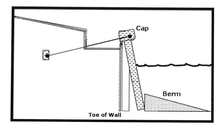
**Symptoms:** Cap rotation, movement or cracking, a gap opening between bulkhead and dock (if present), and support pilings (if present) tight against the bulkhead indicating pressure on the structure from the failure.
