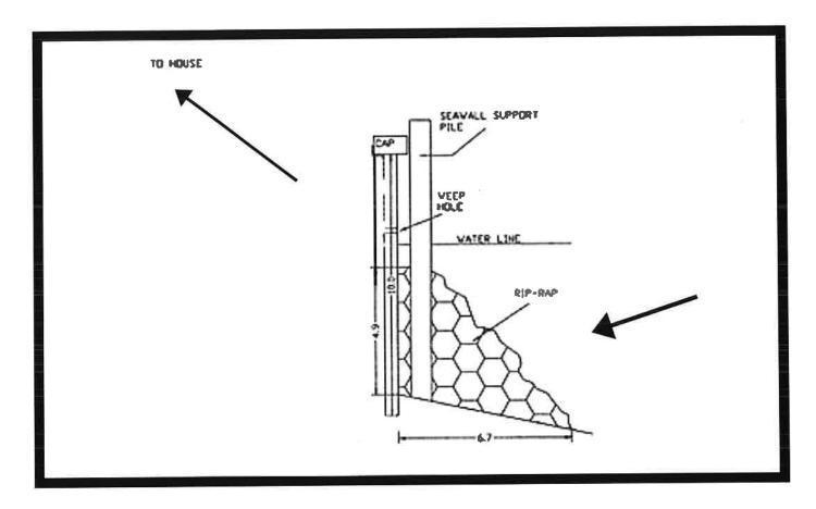
Profile illustration of rip rap. Note degree of necessary protrusion into canal which may make installing a future dock difficult.
