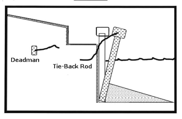
**Symptoms:** A deteriorating cap, wavy or sagging panels, cracks / spalling and backfill settlement.
