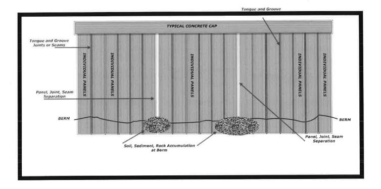
Symptoms: Sinkholes, separation in seams, accumulation of rock, and sediment at base of the affected joint.
