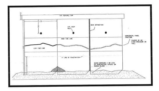
Symptoms: The principal symptom is cracking with rust marks on the panels facing the water.
